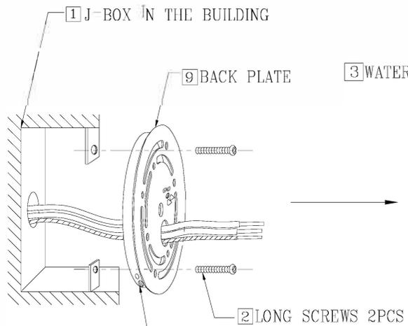
WHEN INSTALL THE FIXTURE, THE THREAD HOLE ON SIDE EDGE OF BACK PLATE SHOULD BE DOWNWARD VERTICALLY.
